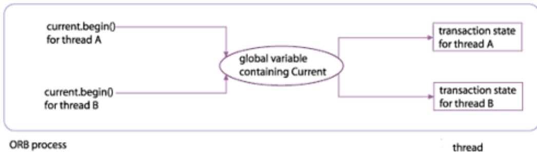
Figure 9 Using a global Current object to start transactions across threads in a process
