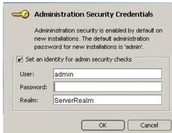
Figure 1 Administration Security Credentials screen with default credential settings
